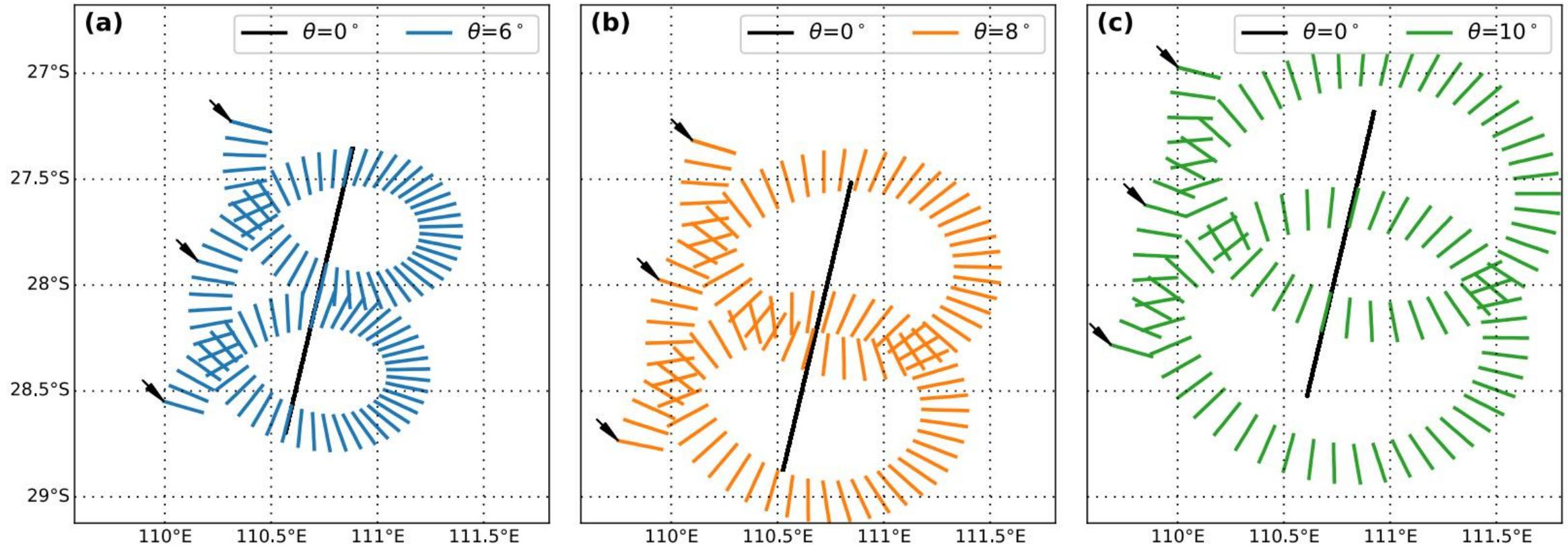
Fig. 1. Example for acquisition pattern of (a) 6°, (b) 8°, and (c) 10° beams within two rotations of 360°. Black curve denotes the footprint of the nadir beam. Note that the slightly varying coverage of these three incidence angles is due to their incontinuous azimuth directions at a given moment. The black arrow indicates the starting position of one entire rotation.
