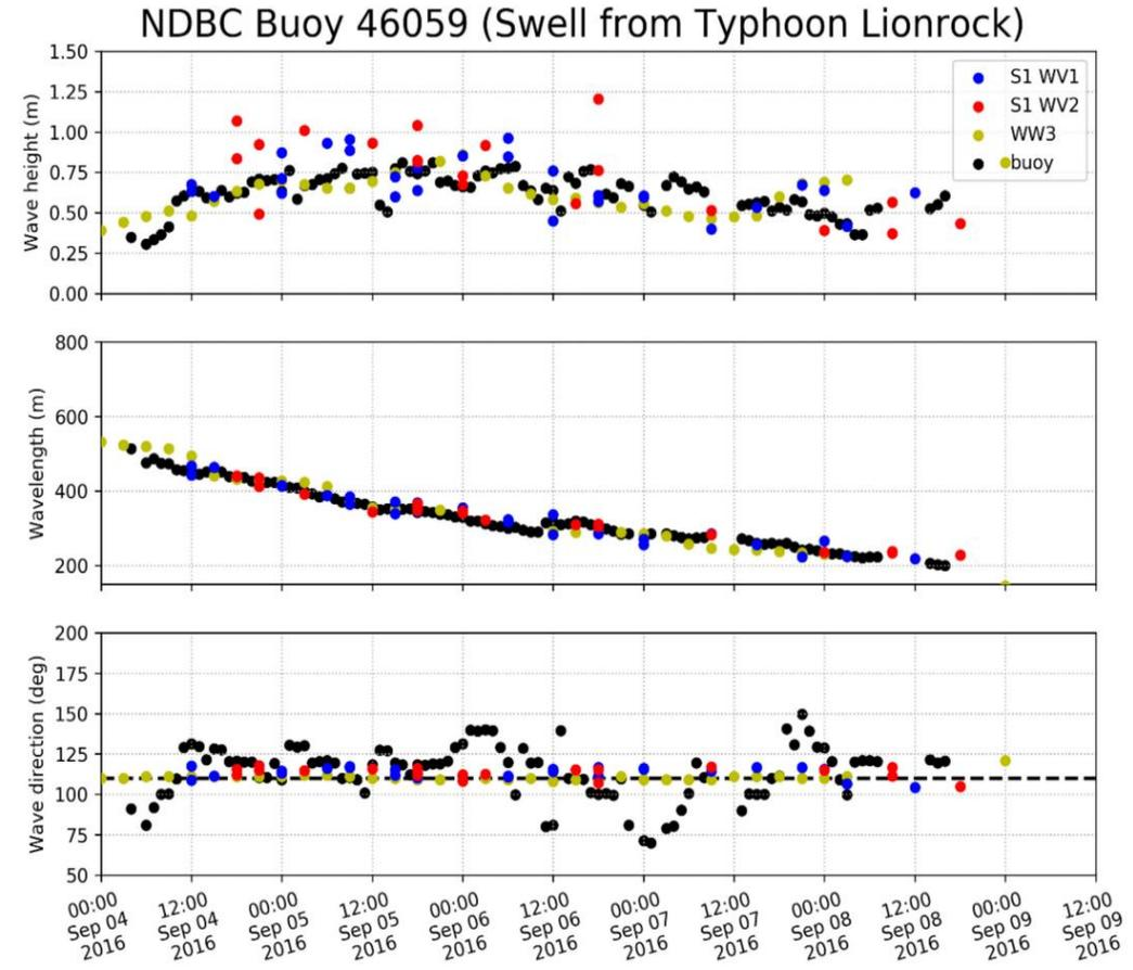
**Figure 17.** As in Figure 16, but for the case of a swell event originated from Typhoon Lionrock on 29 August 2016. The vertical black line corresponds to 12:00:00 UTC 11 September 2016 (the time of buoy observation presented in Figure 7).
