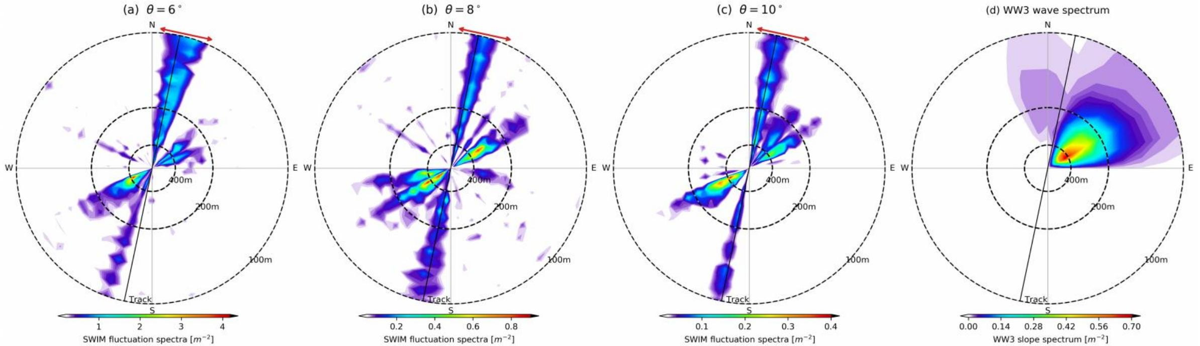
Fig. 4. 2-D fluctuation spectrum constructed from one rotation of  $360^\circ$  for the beam of (a)  $6^\circ$ , (b)  $8^\circ$ , and (c)  $10^\circ$ . (d) Collocated WW3 wave slope spectrum is shown for comparison. The WW3 spectra direction corresponds to the direction that the waves travel to. The red arrow denotes the directional sector where the signal is strong affected by the instrument noise.
