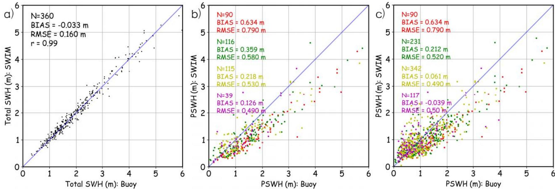
Fig. 12. Comparison of SWH between SWIM 10° beam and buoys. (a) Total SWH. (b) PSWH for best-matched partitions. (c) PSWH for all cross-assigned partitions. The colors of dots and texts in (b) and (c) indicate the number of partitions identified in the collocated buoy spectra (red: one partition, green: two partitions, yellow: three partitions, and purple: four partitions).
