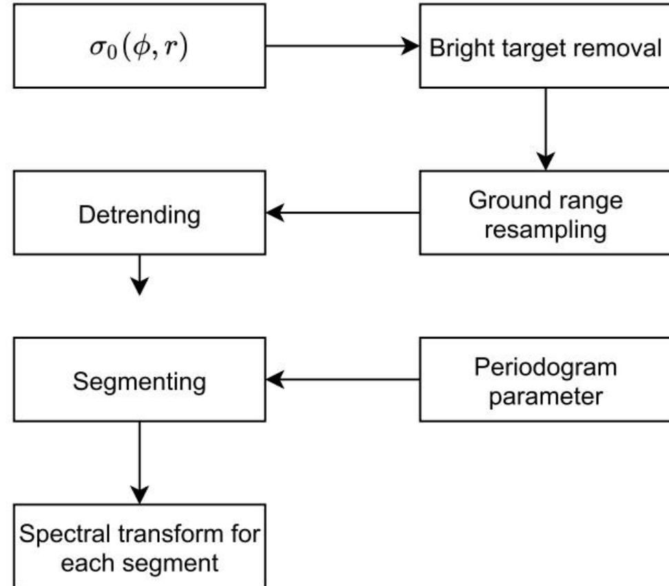
Fig. 2. Flowchart of the fluctuation spectrum estimate along each azimuth direction. The ground-range resampling spacing is set to be 5 m and the periodogram window is 512 pixels with 256 pixels overlapping.
