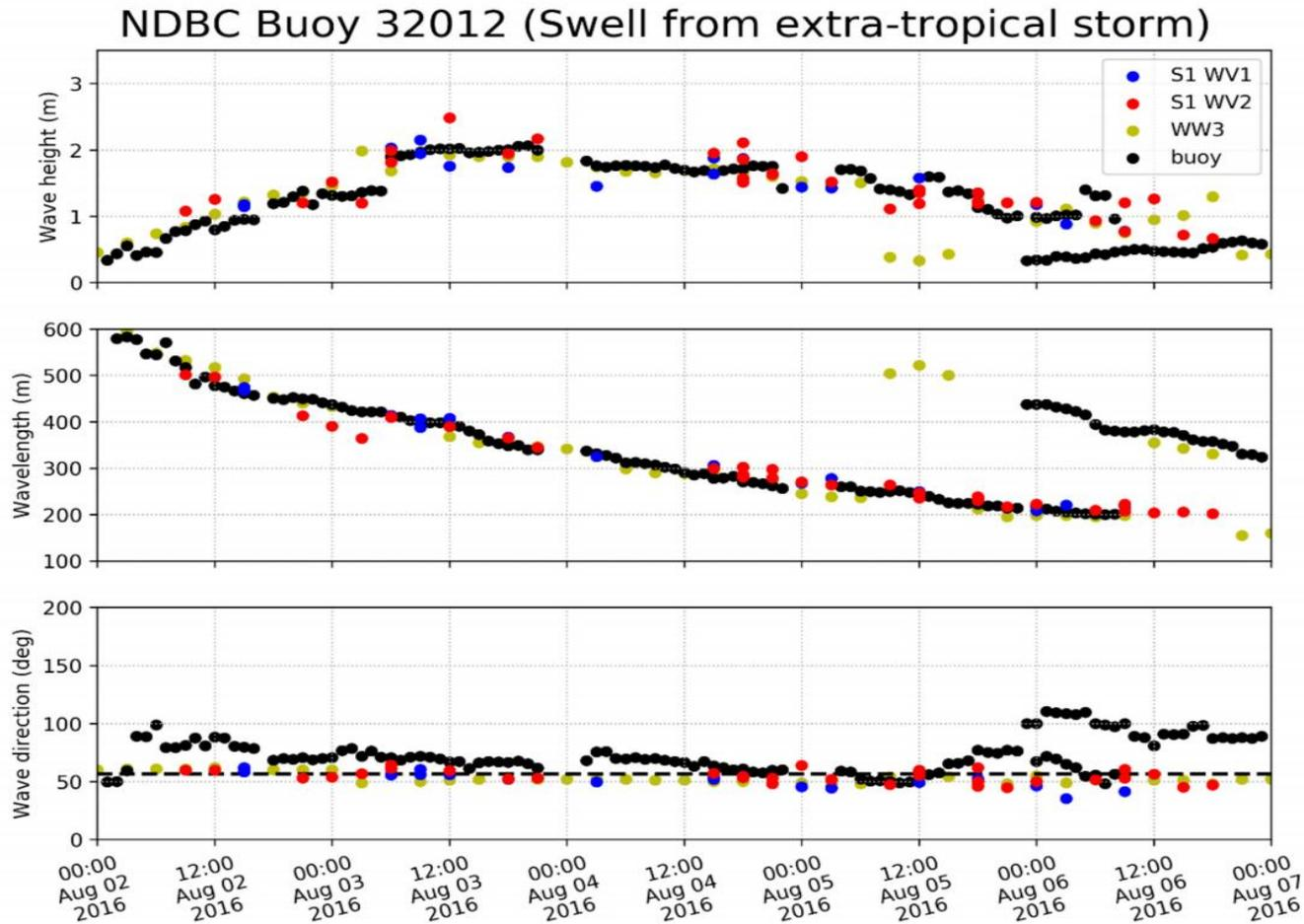
**Figure 16.** Comparison of significant wave height (**top**), peak wavelength (**middle**), and peak direction (**bottom**) from Level-3 CMEMS “fireworks” SAR products (red and blue dots representing Sentinel-1 SAR data in WV1 and WV2, respectively), buoy measurements (black dots) and WW3 model (yellow dots) at the Stratus buoy station #32012 ( $19.63^{\circ}$  S/ $84.95^{\circ}$  W) during the swell event generated by an extra-tropical storm on 28 July 2016.
