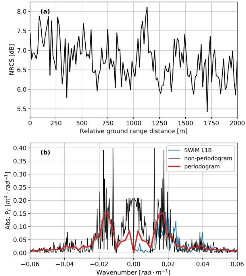
Fig. 3. Example for (a) SWIM measured  $\sigma_0$  profile of  $10^\circ$  beam with respect to the relative ground-range distance. (b) Comparison of the obtained fluctuation spectrum using periodogram algorithm in Fig. 2 (red curve) and nonperiodogram method (black curve) and the results annotated in SWIM level-1B products (blue curve).
