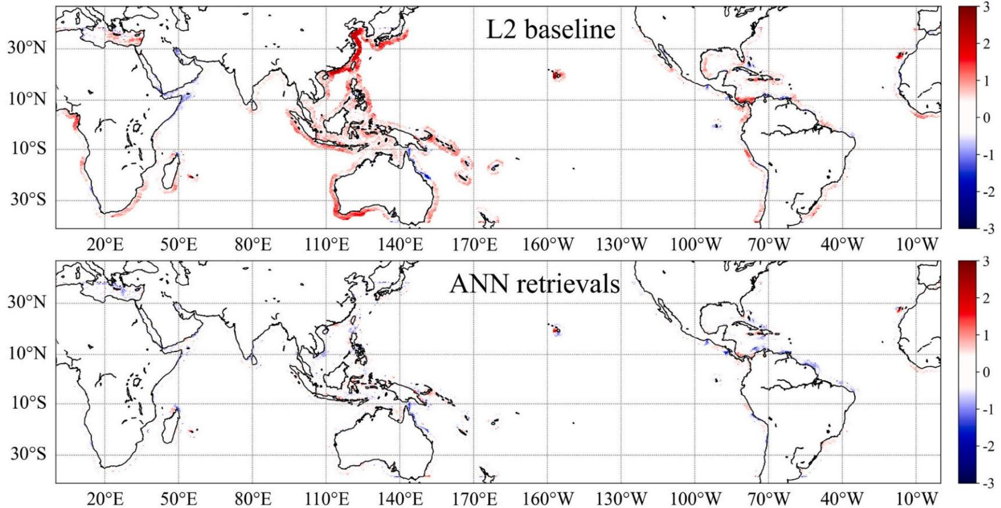
**Fig. 7.** Geographical map of the wind speed biases (CYGNSS wind speed - ERA5 wind speed) along the coastlines. Top: Wind speed bias of the CYGNSS Level 2 v2.1 products. Bottom: Wind speed bias of the ANN based retrieval.
