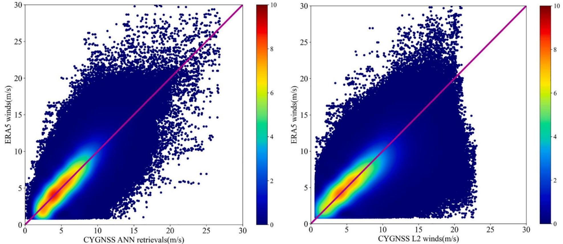
**Fig. 4.** Comparison between the CYGNSS ANN retrieved wind speed and the ECMWF/C3S ERA5 wind speed values (left). Comparison between the CYGNSS baseline L2 v2.1 wind speed and the ECMWF/C3S ERA5 wind speed values (right). The color scale is 1/100000 of the density of points. The purple line shows the 1:1 diagonal. (For interpretation of the references to color in this figure legend, the reader is referred to the web version of this article.)
