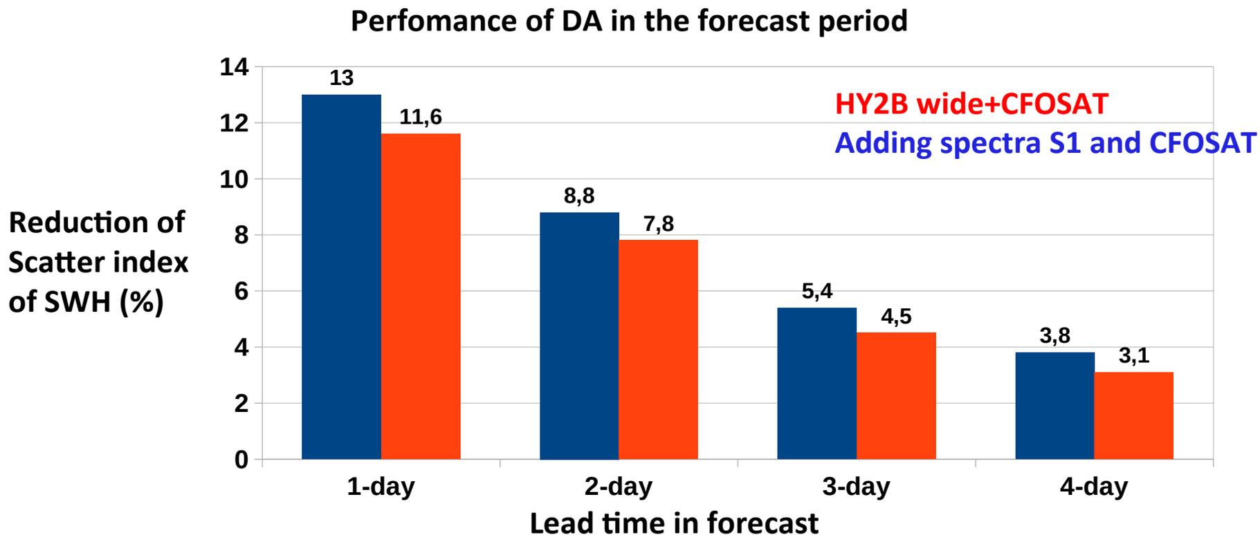
Only two satellite missions with wide swath SWH keep the impact significant after 3 days forecast. The use of directional spectra from S1 and CFOSAT enhances the impact, which remains efficient after 3-day forecast
