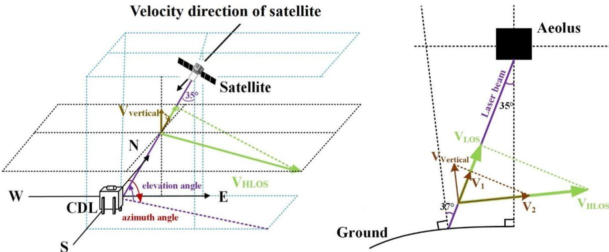
The schematic diagram of the vertical velocity impact on the HLOS velocity retrieval of Aeolus.
