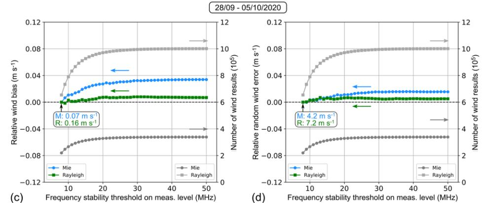
Wind bias (a) and random error (b) of the Mie (blue dots) and the Rayleigh channel (green squares) with respect to the ECMWF model background (O–B) depending on a frequency stability threshold for the period between 17 and 24 August 2020. Panels (c) and (d) show the corresponding data for the week between 28 September and 5 October 2020.
