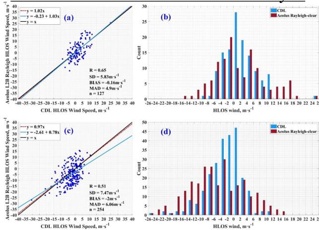
Comparisons of Aeolus Rayleigh-clear HLOS against the CDLretrieved HLOS according to the measurements made on (a)(b) ascending and (c)(d) descending tracks.
