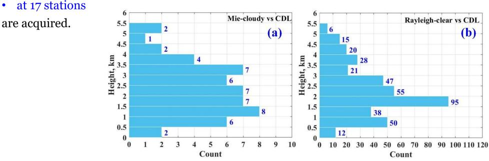
Counts of data pairs at different height ranges of (a) Mie-cloudy vs CDL and (b) Rayleigh-clear vs CDL
