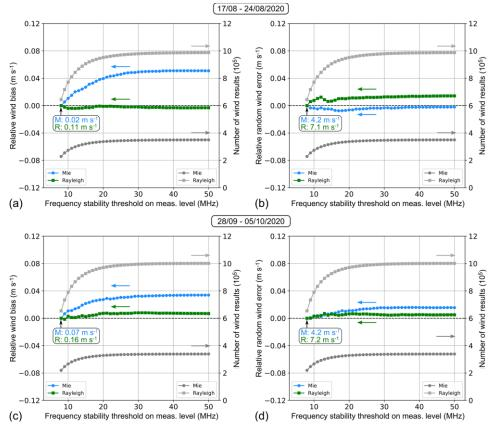
Wind bias (a) and random error (b) of the Mie (blue dots) and the Rayleigh channel (green squares) with respect to the ECMWF model background (O–B) depending on a frequency stability threshold for the period between 17 and 24 August 2020. Panels (c) and (d) show the corresponding data for the week between 28 September and 5 October 2020.
