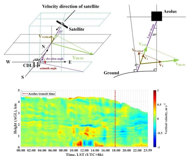
The schematic diagram of the vertical velocity impact on the HLOS velocity retrieval of Aeolus.
