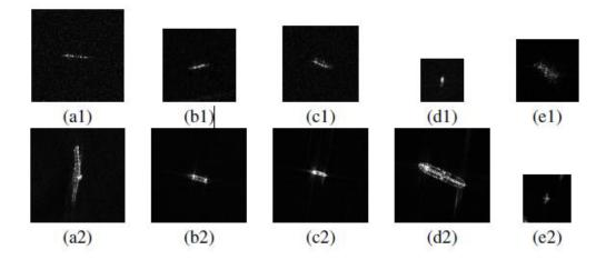
Fig. 2. Each class in the two datasets. The first row is from OpenSAR and the second row is from FUSAR. (a) Cargo. (b) Dredging. (c) Fishing. (d) Tanker. (e) Others.
