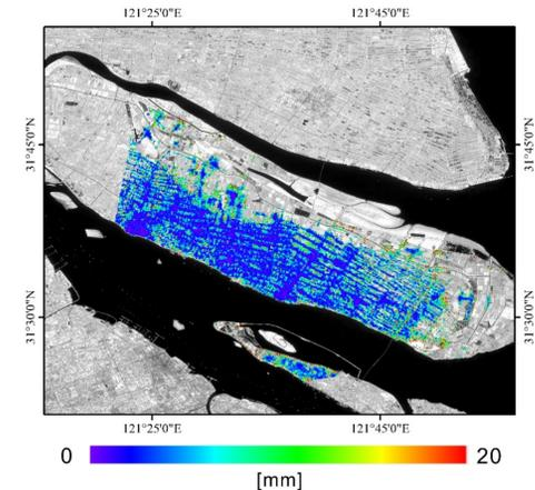
Figure. 3 Combination error distribution of RST-2MF, RST-2W and S1A.
