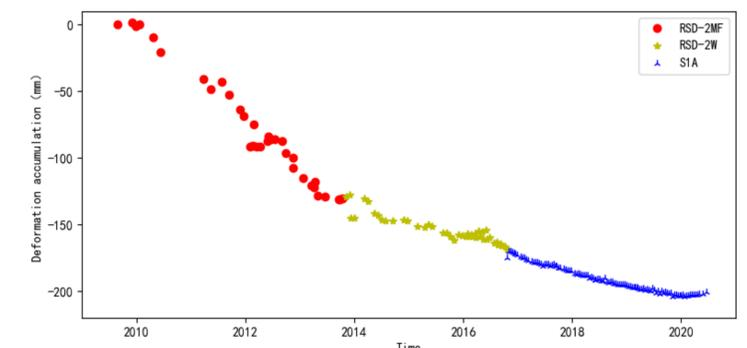
Figure. 4 The plots of combine deformation time-series at the point with maximum deformation during the 2009-2020 in Chongming Island.
