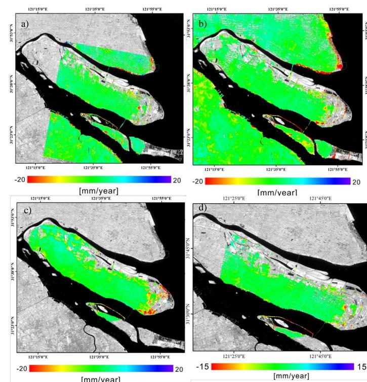
Figure. 2 Geocoded map of the mean (vertical) deformation velocity of Chongming Island, as retrieved by a) RST-2MF vertical deformation time-series during the 2009-2013, b) RST-2W vertical displacement time-series during the 2012-2016, c) S1A vertical deformation time-series during the 2015-2020, d) combining RST-2MF, RST-2W and S1A vertical deformation time-series during the 2009-2020.
