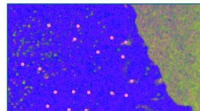
Detections with Gaussian CFAR filters using product (blue), and sum (purple) of the HV/HH bands
