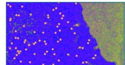
Objects detected with iterative (yellow), and Wishart-based (violet) CFAR filters
