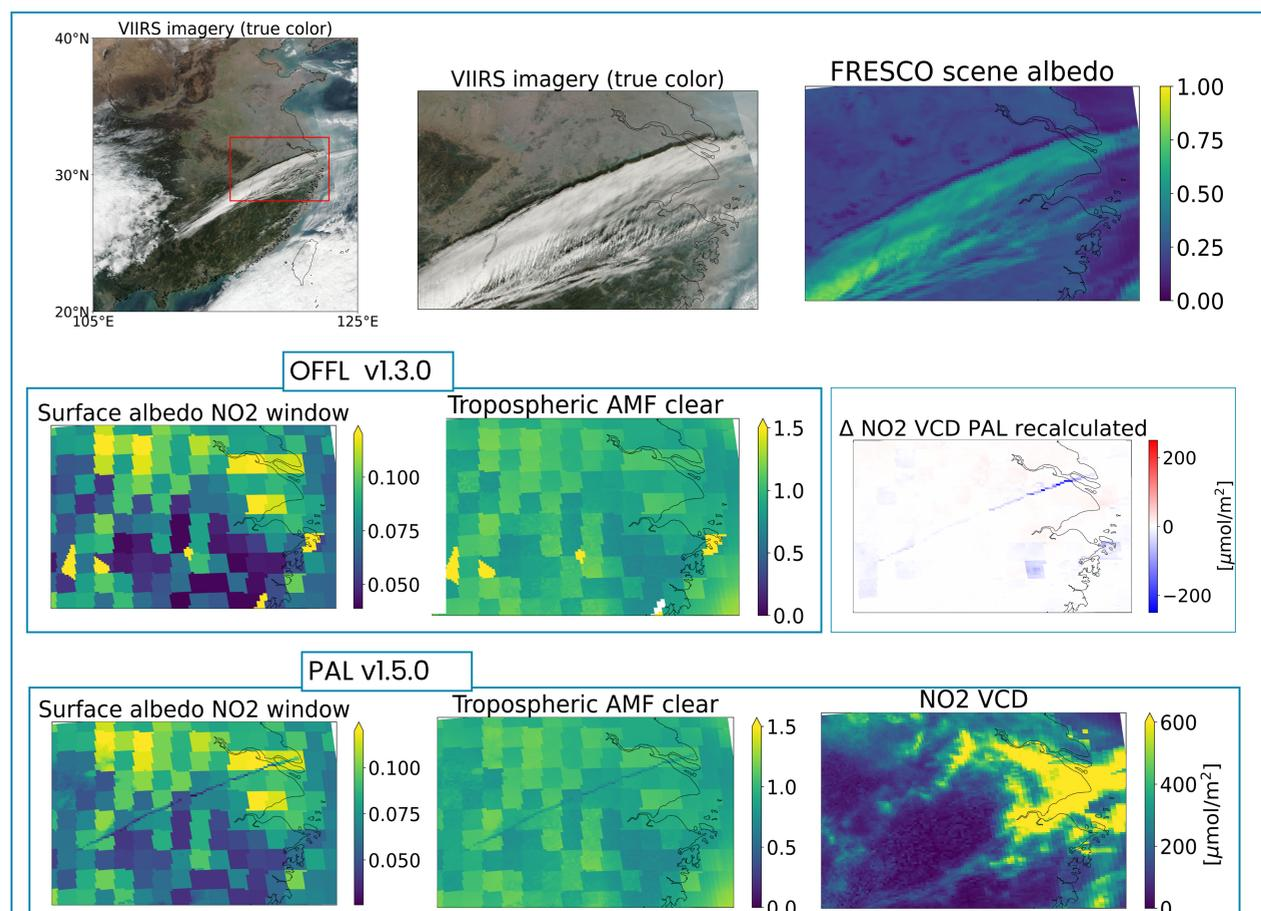
Figure 2: Cloud shadow in Shanghai area on 04-12-2019 in the S5P NO<sub>2</sub> PAL and OFFL products. The pixel size is 5.6x3.6 km<sup>2</sup>.
