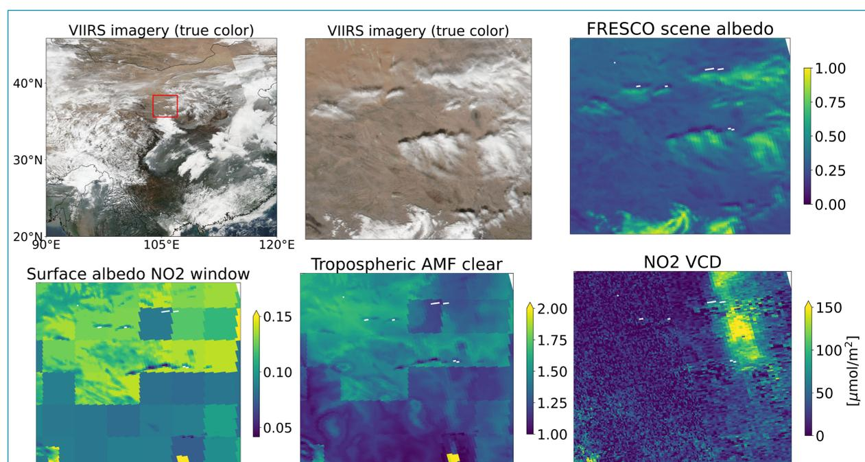
Figure 1: Cloud shadow in Gansu province on 03-03-2018 in the S5P NO<sub>2</sub> zoom data-set. The pixel size is 2.4x1.8 km<sup>2</sup>, increasing here towards the East-side of the orbit due to the alternative binning scheme.
